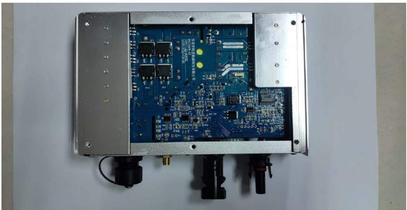
Photo 6 - Internal view of the unit, model WVC-300, WVC-350
